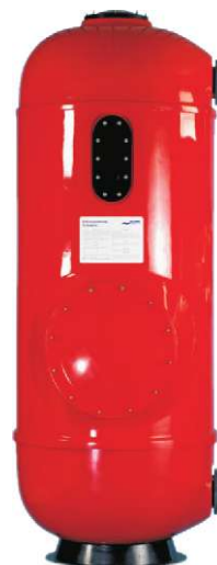
KOK DIN: filtration bed 1,2 m, collector plate with PVC nozzles, diameters: 610 mm, 765 mm, 920 mm, 1080 mm, 1250 mm.
